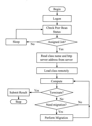
Fig. 8. Working process of a client.
