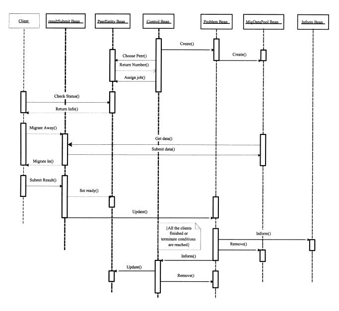
Fig. 9. Working process of server.
